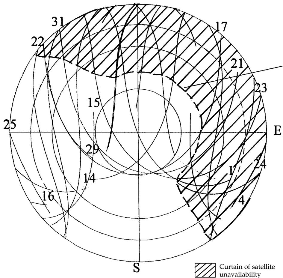
**Fig. 3.** Computer output from the GPS software showing the position of the satellites given certain threshold levels for the topography. The output is for Hardys Bay and shows that satellites 25, 15, 29, 14 and 16 are available in the western sky on that day. The threshold elevation was 15 degrees and 27 satellites were considered.
