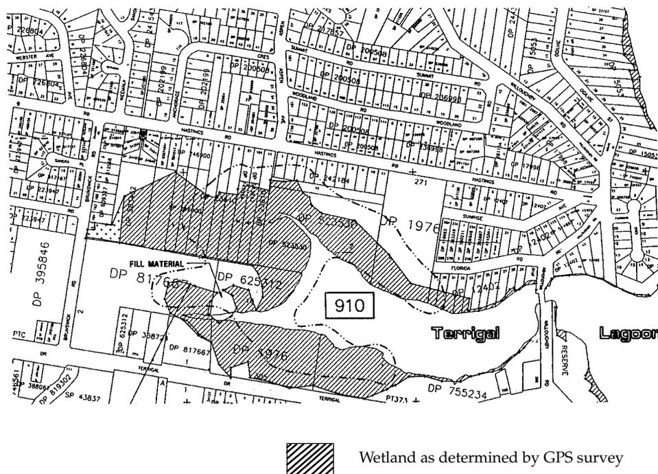
Fig. 4. Terrigal Lagoon showing the SEPP 14 boundary ( - - - - ) and the same boundary determined by GPS survey. Note there are large differences in position.
